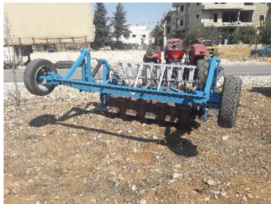
Figure 2: Imprinter designed by the project to be used for rangeland rehabilitation interventions
